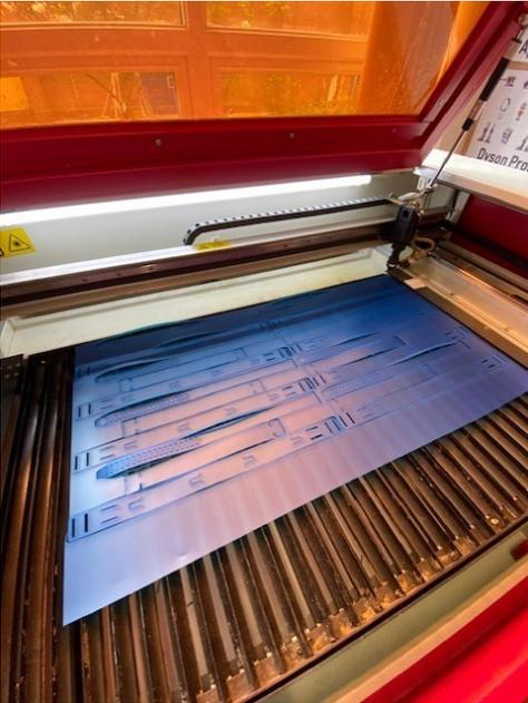
The CAD file consists of three different parts: a headband, forehead spacer and an adjustable strap, which are cut from a thin, flexible plastic called polypropylene. A clear PVC sheet is then hand cut to clip into place on the headband. The benefits of both these plastics are that they have good chemical resistance,
