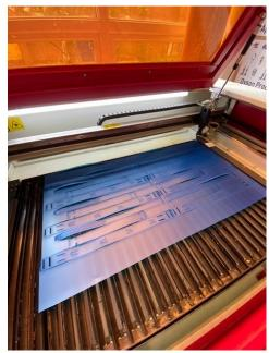
The CAD file consists of three different parts: a headband, forehead spacer and an adjustable strap, which are cut from a thin, flexible plastic called polypropylene. A clear PVC sheet is then hand cut to clip into place on the headband. The benefits of both these plastics are that they have good chemical resistance,
